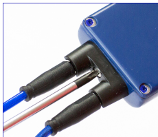
I. Unscrew Connectors Locking Clip (CLC)
